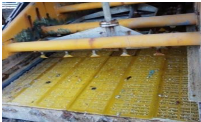
Photo 6: Processus du criblage
