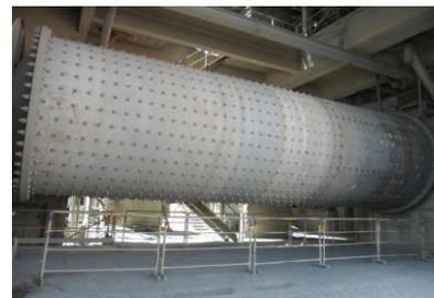
Figure 11 : Broyeur cuite (broyeur ciment)
